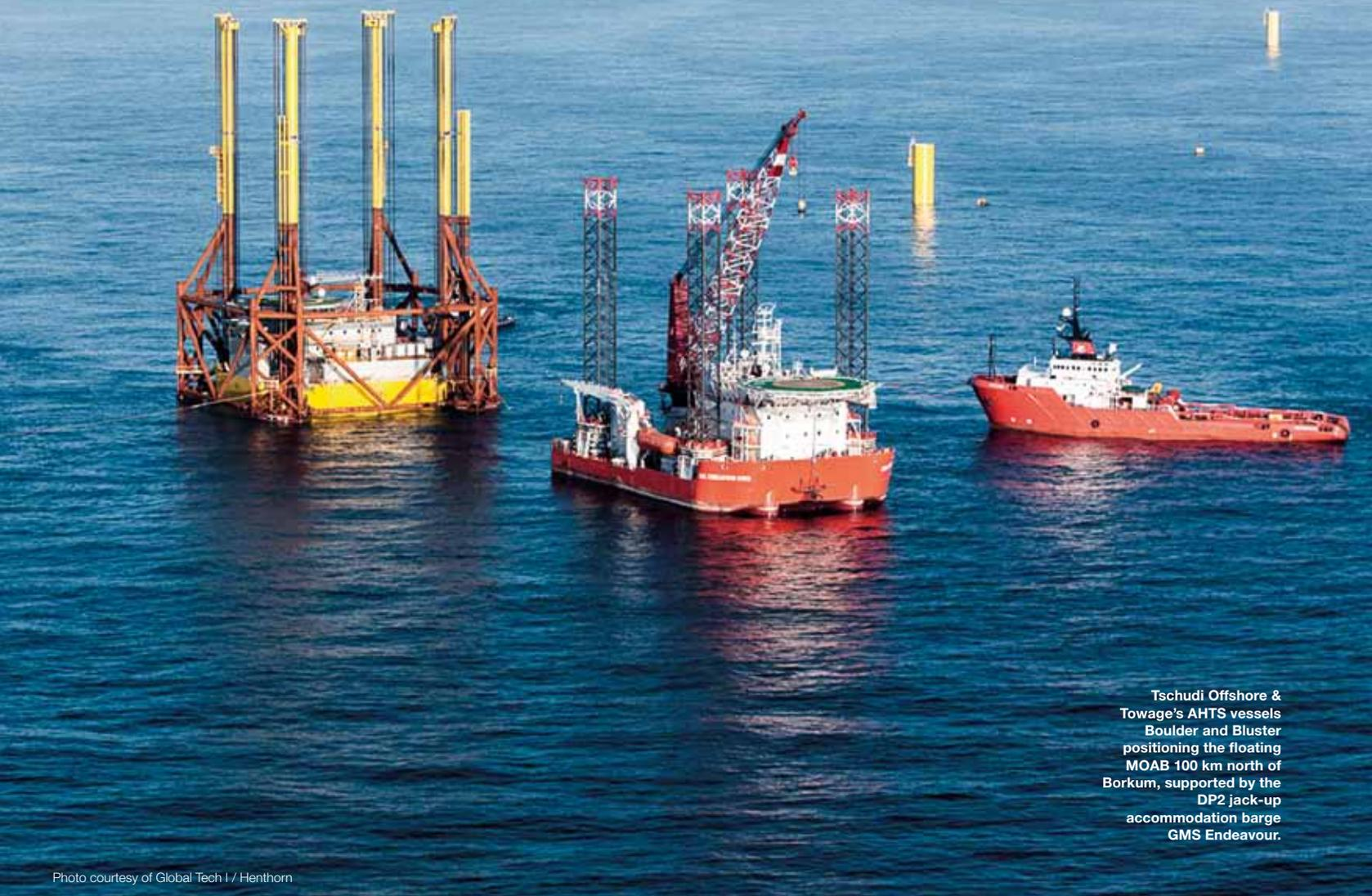
Tschudi Offshore & Towage's AHTS vessels Boulder and Bluster positioning the floating MOAB 100 km north of Borkum, supported by the DP2 jack-up accommodation barge GMS Endeavour.
