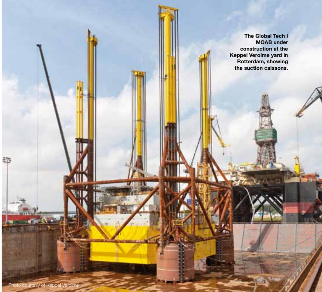
The Global Tech I MOAB under construction at the Keppel Verolme yard in Rotterdam, showing the suction caissons.
